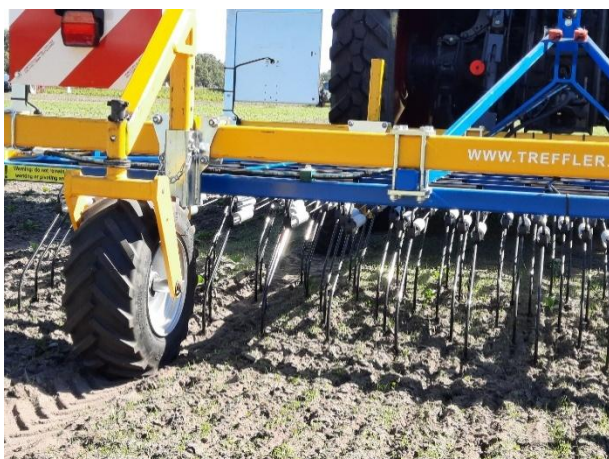
Figure 24 Mechanical weeding with Treffler harrow, source: Delphy
