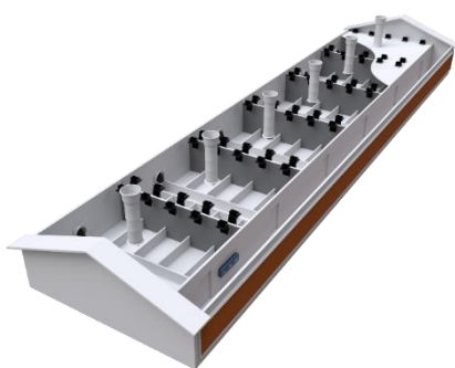
Figure 10 Illustration of ventilation system. Source: SKOV A/S
