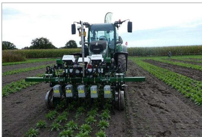
Figure 23 Mechanical weeding with Garfield, source: Delphy
